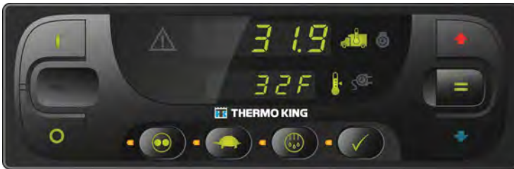
Figure 11. Truck Standard Display HMI Control Panel
